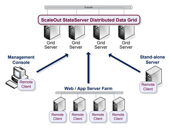
The distributed data grid would hold shopping carts to efficiently handle a large workload of online shopping traffic, while a backend database server stores completed transactions, inventory, and customer records.
